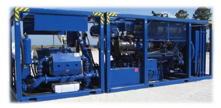
The **FPS-1350** is a skid mounted pumper rated to a maximum working pressure of 10,400 psi and 1,150 HHP. The 8 manual transmission makes the unit capable of delivering steady pump rates from 0.25 bpm to 8 bpm.
