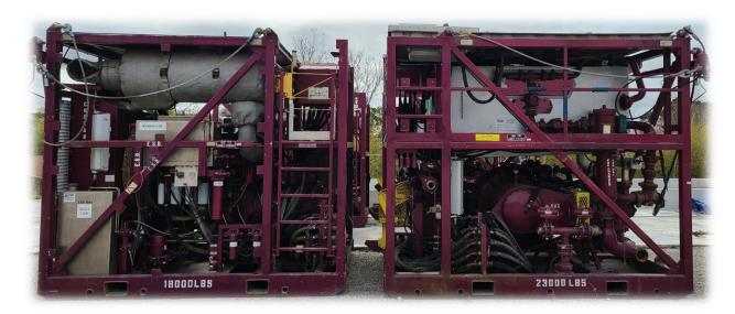
The FPS-600 is a skid mounted pumper rated to a maximum working pressure of 11,315 psi and 600 HHP. The 8 manual transmission makes the unit capable of delivering steady pump rates from 0.25 bpm to 6 \(^3\)4 bpm.
